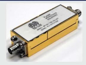
PMI Model BP13G-10G-CD-SFF is a suspended substrate bandpass filter that offers a wide passband of 8 to 18GHz. This filter offers a low insertion loss of 1.5dB typically and a passband VSWR of 2.0:1 maximum. Stopband rejection of 70dB typical is provide from DC to 6GHz and from 20 to 23GHz. This model is offered with field removable SMA connectors so it can be used in connectorized form or as a drop-in module. The size is 1.94" x 0.76" x 0.5".
